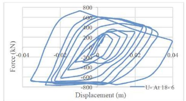
**Figure 31:** The force-displacement curve of the U-At 18-6 model.
