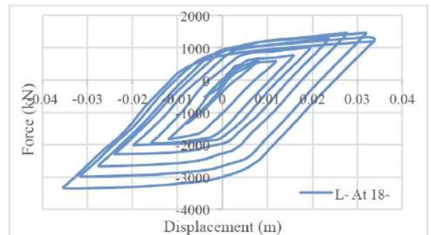
Figure 20: The force-displacement curve of the L-At 18-8 model.
