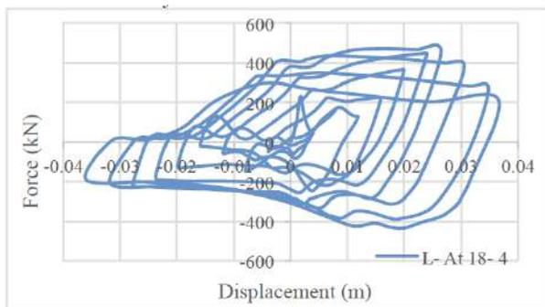
Figure 18: The force-displacement curve of the L-At 18-4 model.
