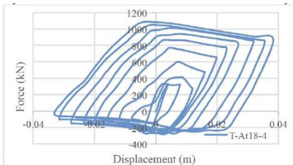
Figure 24: The force-displacement curve of the T-At 18-4 model.
