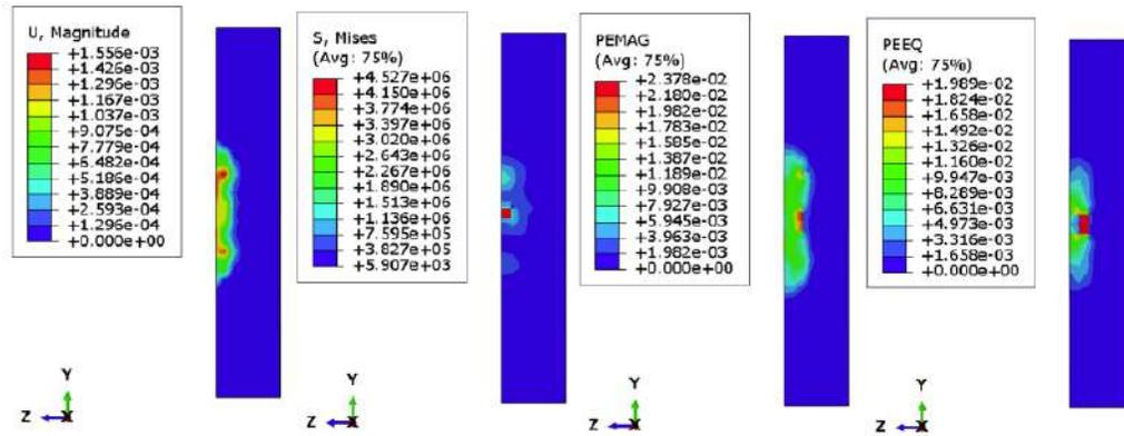
Figure 15: The graphic outputs of concrete in the model with a T-shaped stud.
