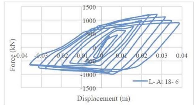
Figure 19: The force-displacement curve of the L-At 18-6 model.
