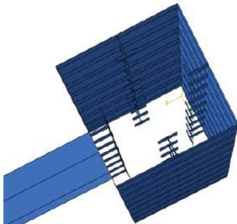
**Figure 7: Internal view of shear studs.**
