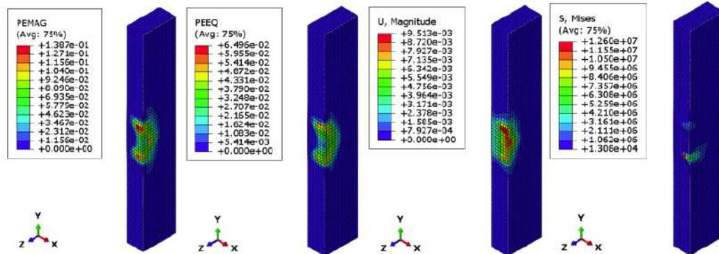
Figure 16: The graphic outputs of concrete in the model with a U-shaped stud.
