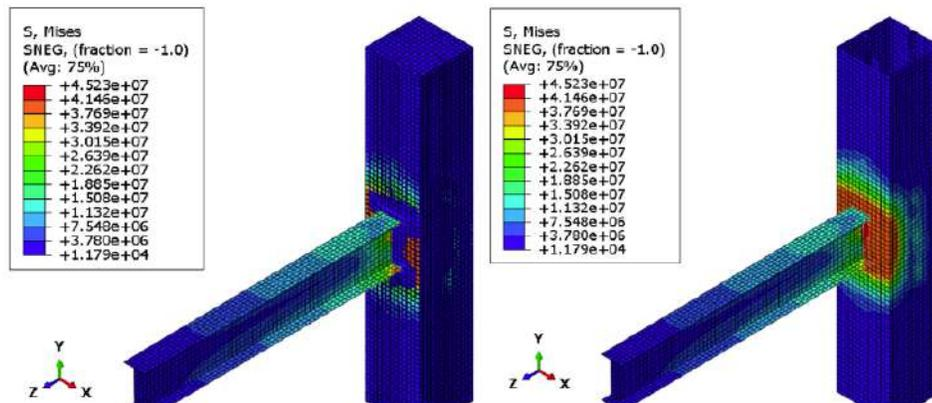
Figure 14: The stresses in the model with L-shaped studs.
