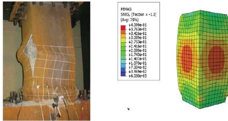
Figure 3: Comparing the maximum plastic strains in the numerical model with experimental model.
