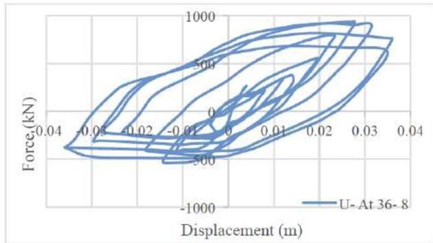
**Figure 35:** The force-displacement curve of the U-At 36-8 model.
