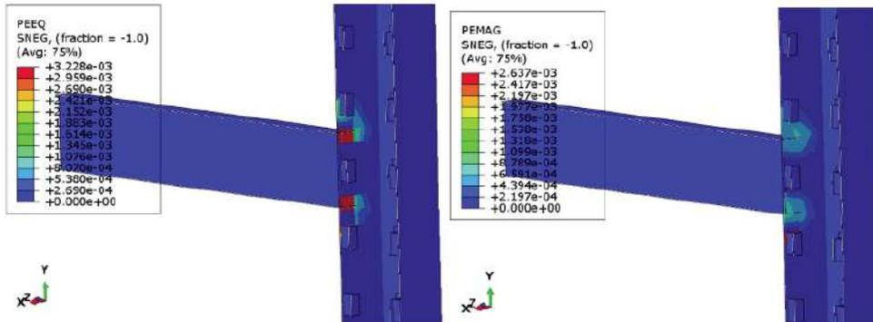
Figure 9: Display of plastic strains in models with T-shaped studs.
