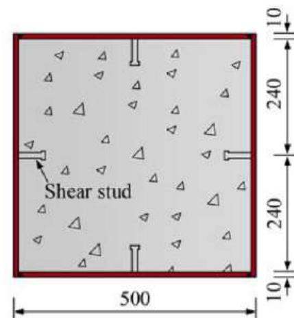
**Figure 2:** Section of the validation model (Wang *et al.*, 2019).
