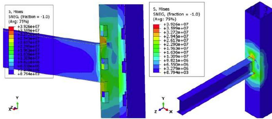
Figure 12: The stresses in the model with T-shaped studs.
