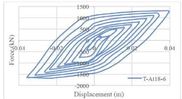
Figure 25: The force-displacement curve of the T-At 18-6 model.
