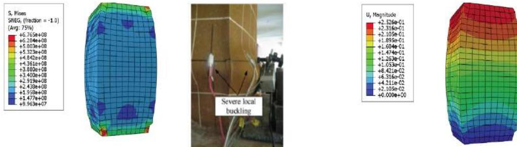
Figure 5: Comparing the maximum stress and displacement in the numerical model with experimental model.
