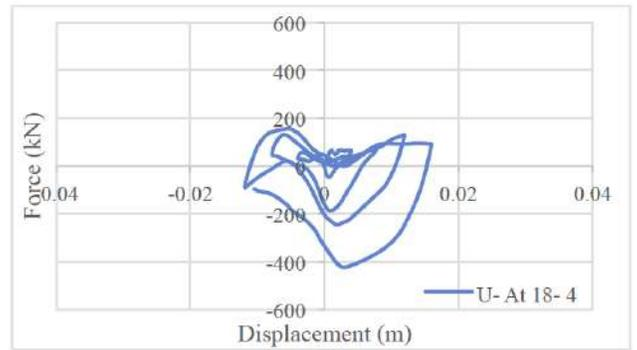
**Figure 30:** The force-displacement curve of the U-At 18-4 model.
