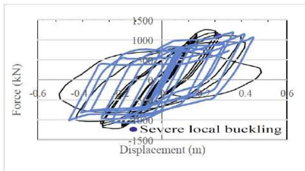
Figure 6: Comparison of the force-displacement diagram of the experimental SC-1-0.4 model with the validation numerical model.
