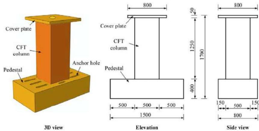
**Figure 1:** Geometry and dimensions of the validation model (Wang *et al.*, 2019).
