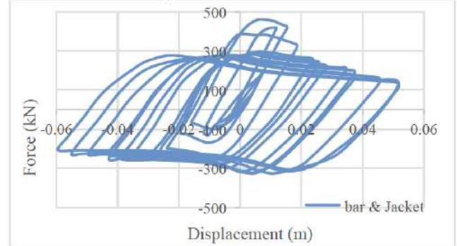
**Figure 36:** The force-displacement curve of the model without shear stud.
