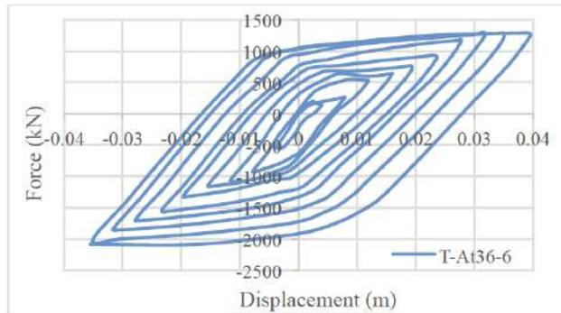
**Figure 28:** The force-displacement curve of the T-At 36-6 model.
