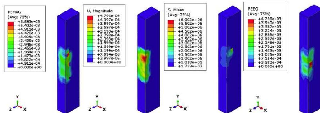
Figure 17: The graphic outputs of concrete in the model with a L-shaped studs.
