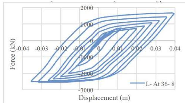
Figure 23: The force-displacement curve of the L-At 36-8 model.
