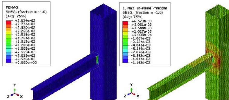
Figure 10: The strains in the models with L-shaped studs.
