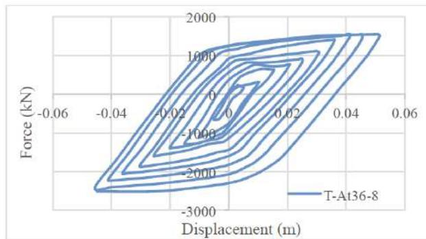
**Figure 29:** The force-displacement curve of the T-At 36-8 model.
