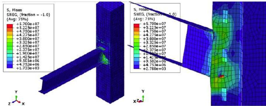
Figure 13: The stresses in the model with U-shaped studs.
