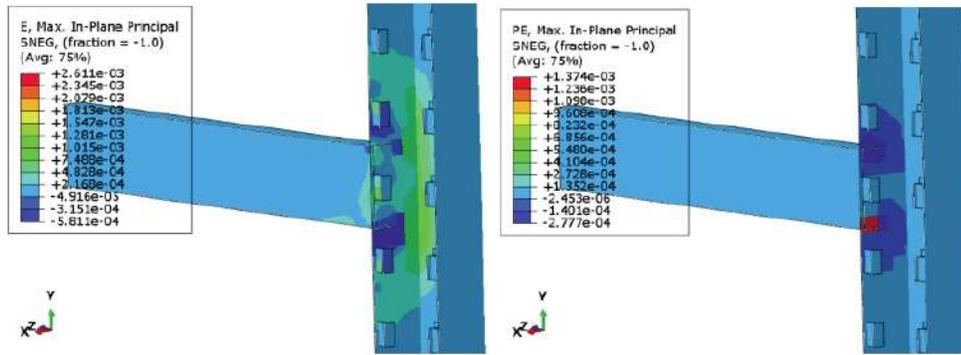
Figure 8: Display of elastic strains in models with T-shaped studs.
