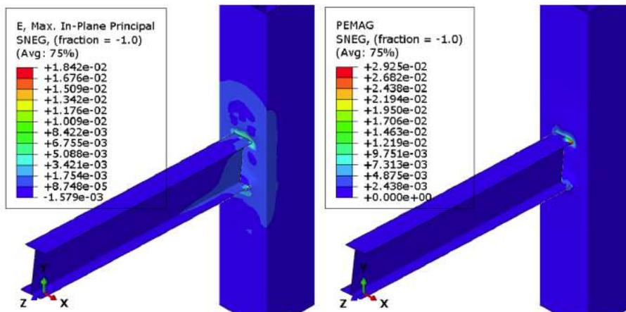
Figure 11: The strains in the models with U-shaped studs.
