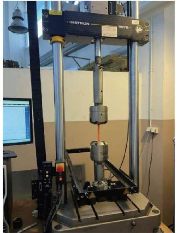
**Figure 3:** Instron 8872 with sample mounted.
